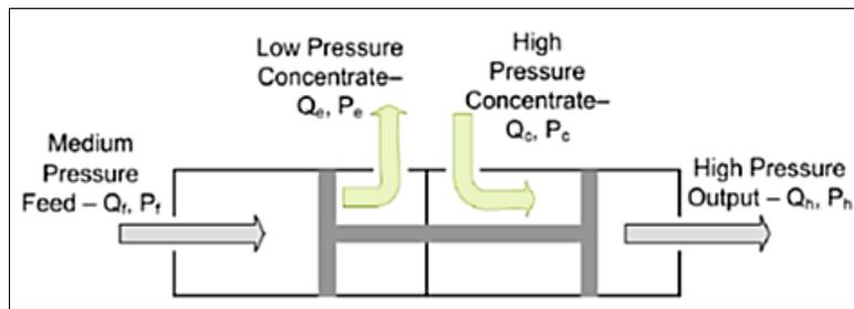
Fig. 5. Basic pump mechanics [5].
