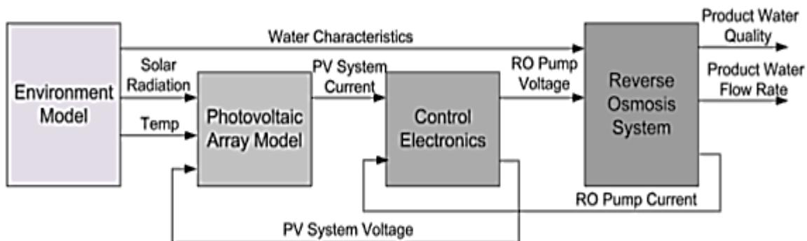
Fig. 4. PVRO model in MATLAB/ Simulink [8].
