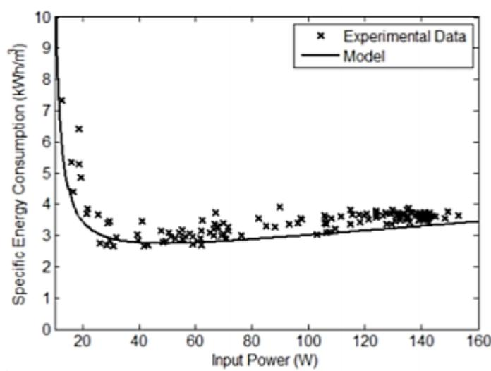
Fig. 10. Overall efficiency of RO system [8].
