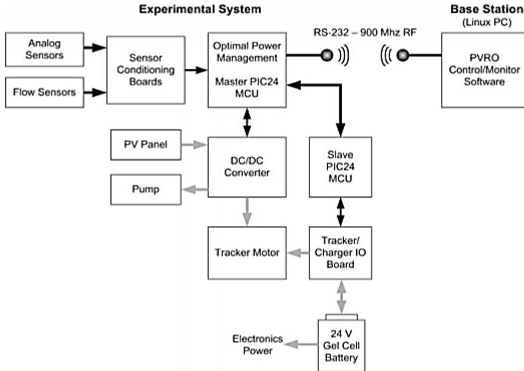
Fig. 7. Experimental system architecture [8, 9].
