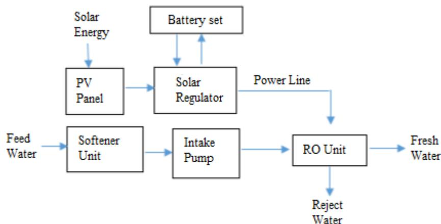
*Fig. 2. Block diagram of the system [5].*
