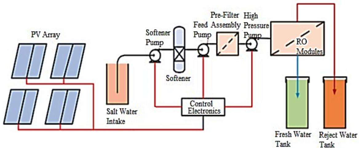
Fig. 3. Photovoltaic reverse osmosis (RO) system flow diagram [5].
