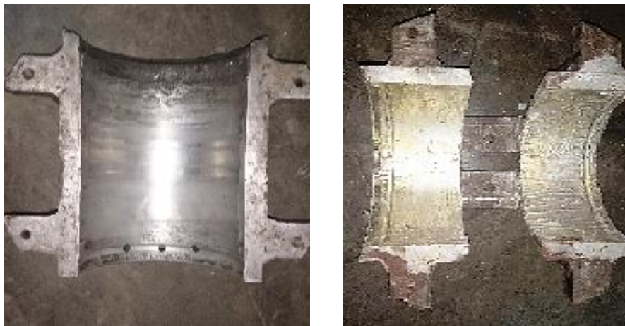
Fig. 1. An effect of metal to metal contact due to whirl phenomenon.
