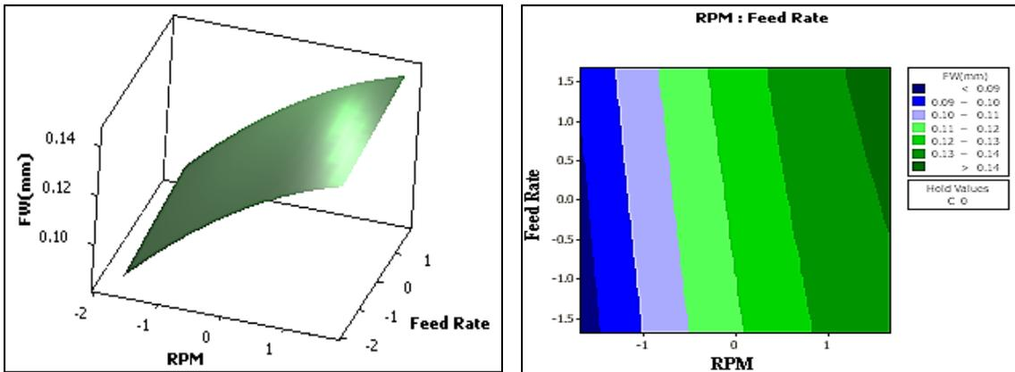
Fig. 7. Variation in Tool Wear According to Change in RPM and Feed Rate.
