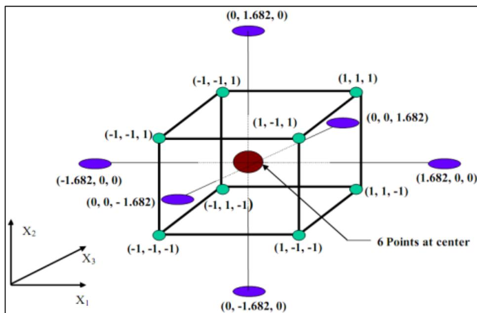
**Fig. 3.** Central Composite Rotatable Design in 3X-Variables (Cochran and Cox, 1962).
