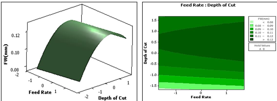
Fig. 8. Variation in Tool Wear According to Change in Feed Rate and Depth of Cut.
