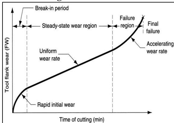
Fig. 2. Different Stages of Wear.
