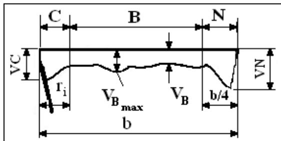
Fig. 1. Flank Wear.
