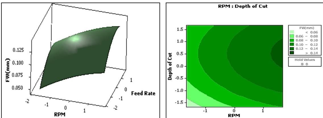
Fig. 9. Variation in Tool Wear According to Change in RPM and Depth of Cut.
