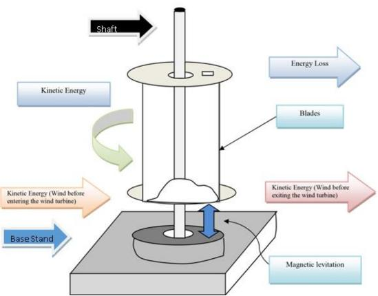
Fig. 3. Components of a Maglev turbine.
