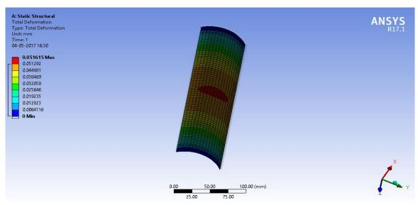
Fig. 4. Total Deformation of Blade.
