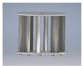
Fig. 9. Turbine model in inventor.
