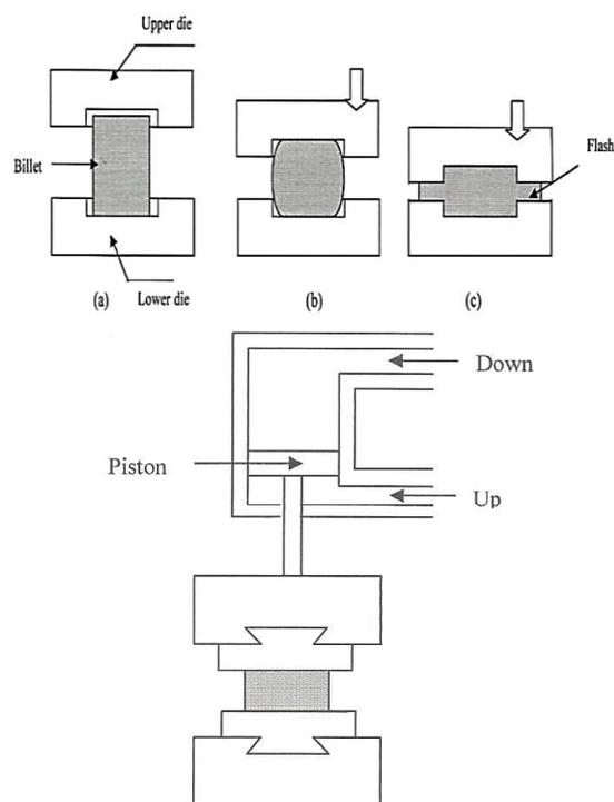
**Fig. 2.** Forging operation.
