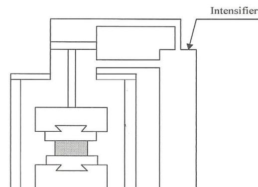
**Fig. 3.** Closed die forging.
