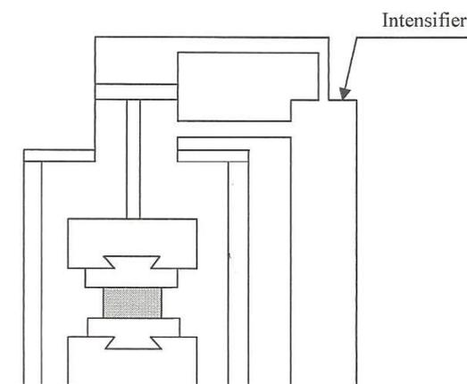
Fig. 4. Forging intensifier.
