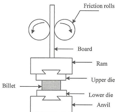
**Fig. 1.** Open die forging.
