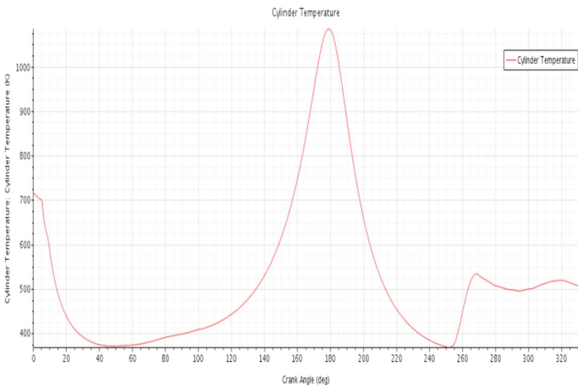
Figure 17. (c) Temperature vs Crank Angle at 2000 rpm.
