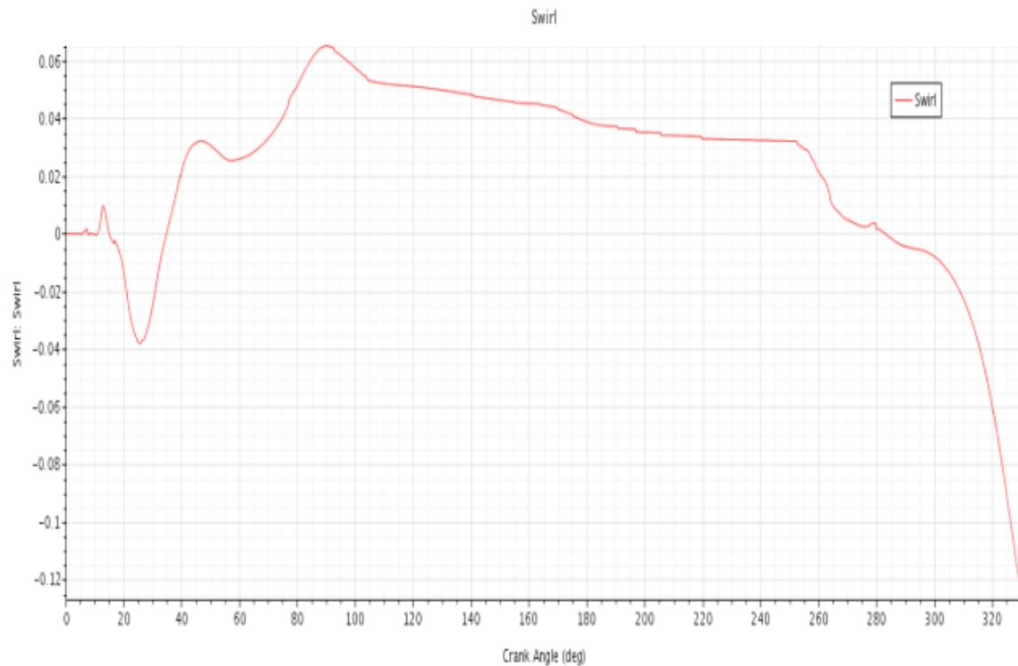
**Fig 19 (d)** Swirl vs Crank angle at 3000 rpm.
