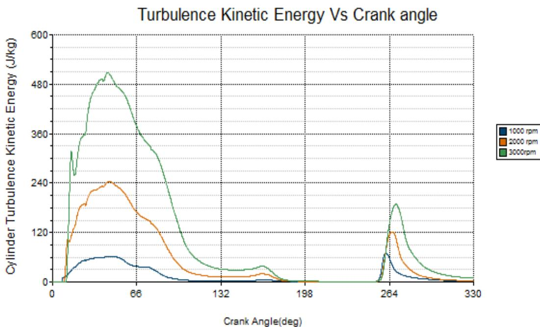
**Figure 18.** (a) Variation of Turbulent Kinetic Energy with respect to crank angles at Various speeds.
