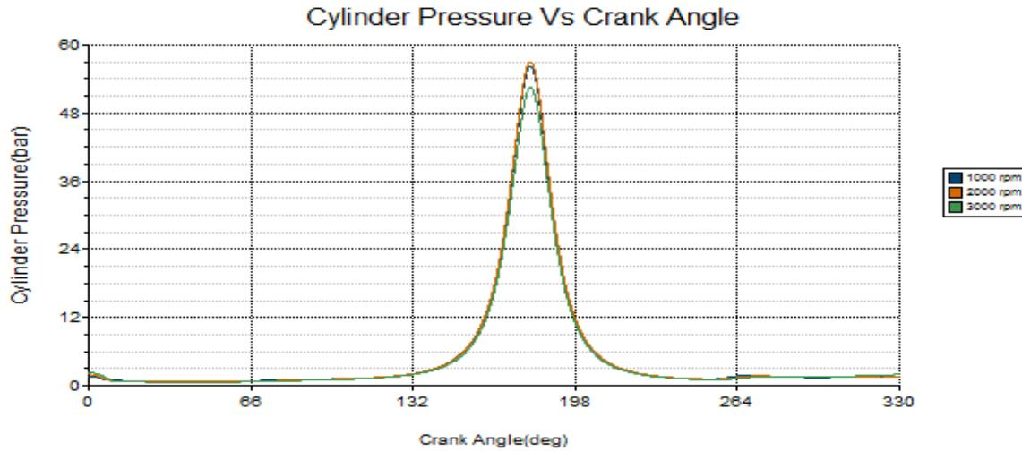
**Figure 16.** (a) Variation in the cylindrical pressure with respect to crank angle at various speeds.
