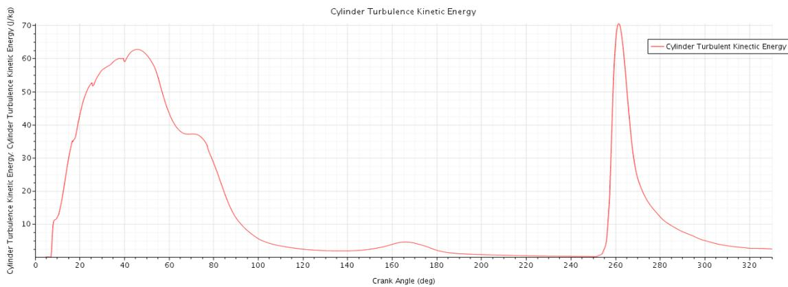
**Figure 18. (c)** Turbulent kinetic energy vs crank angle at 2000 rpm.
