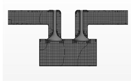
**Figure 3.** (c) Mesh is generated during compression process when both the valves are closed.
