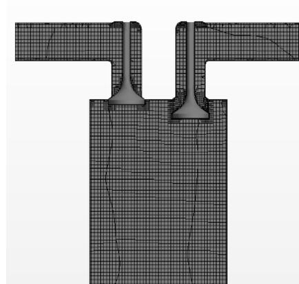
**Figure 3.** (e) Mesh is generated during exhaust process when the exhaust valve opens.
