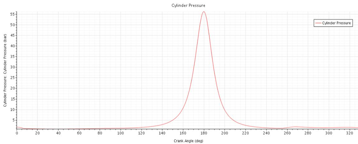
**Figure 16.** (b) Pressure vs Crank angle at 1000 rpm.
