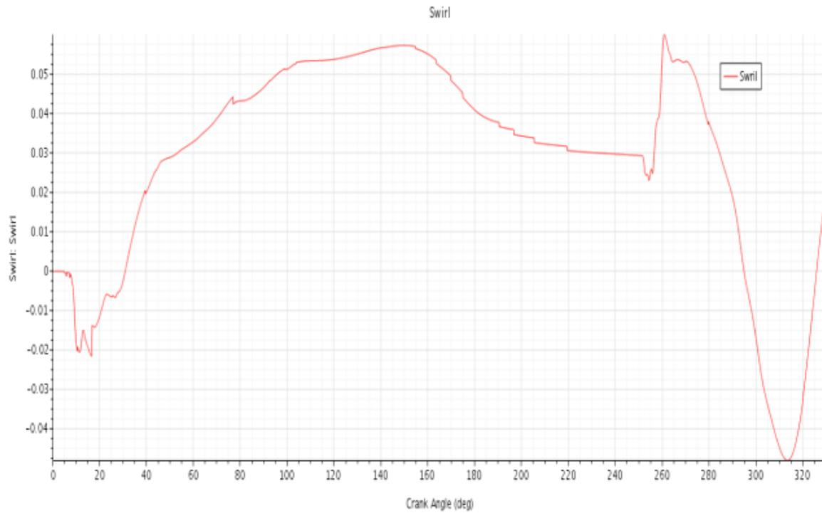
**Figure 19.** (c) Swirl vs Crank angle at 2000 rpm.
