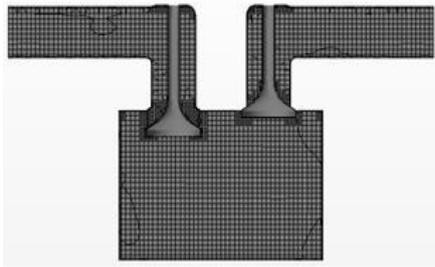
**Figure 3.** (b) Mesh is generated during suction process when the inlet valve opens.
