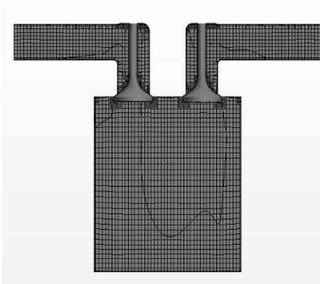
**Figure 3.** (d) Mesh is generated during expansion process when both the valves are closed.
