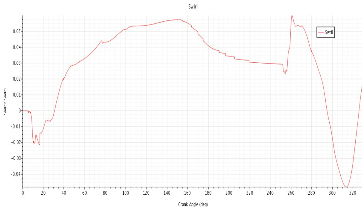
Figure 19. (b) Swirl vs Crank angle at 1000 rpm.
