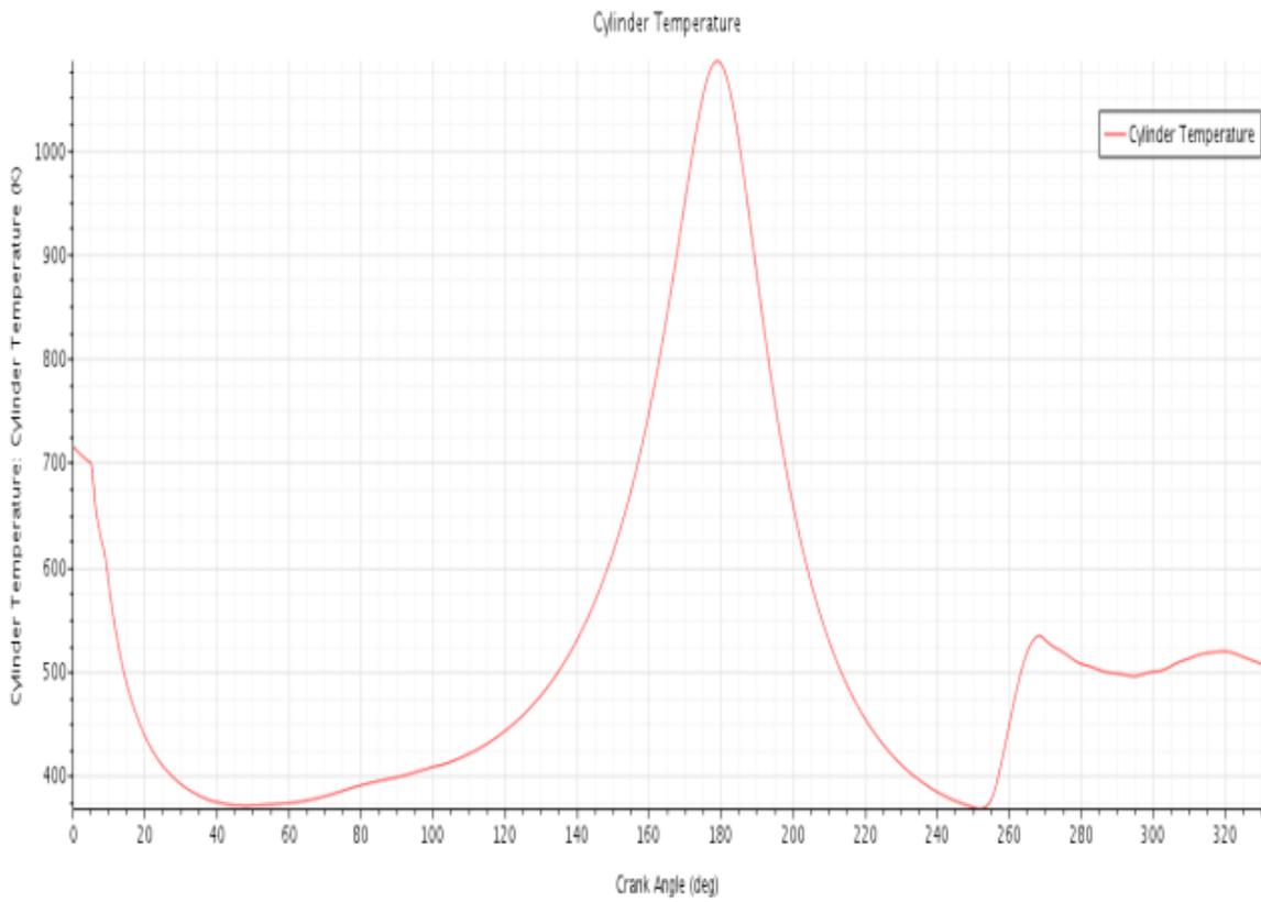
Figure 17. (b) Temperature vs crank angle at 1000 rpm.
