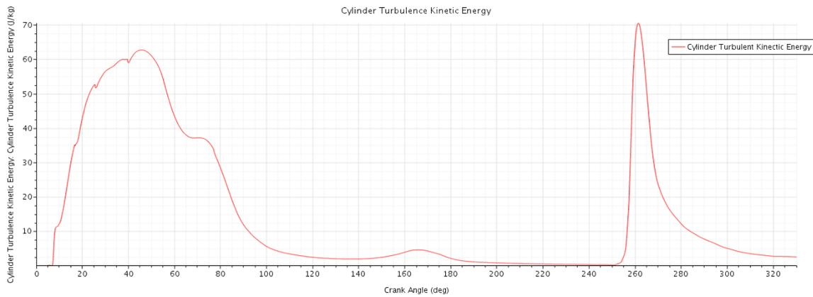
**Figure 18. (b)** turbulent kinetic energy vs crank angle at 1000 rpm.
