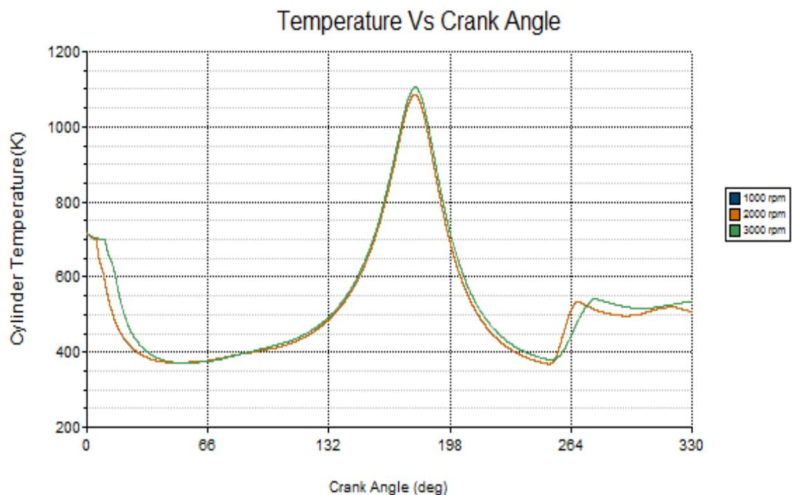
**Figure 17.** (a) Variation of temperature with respect to the crank angle at three different speeds.
