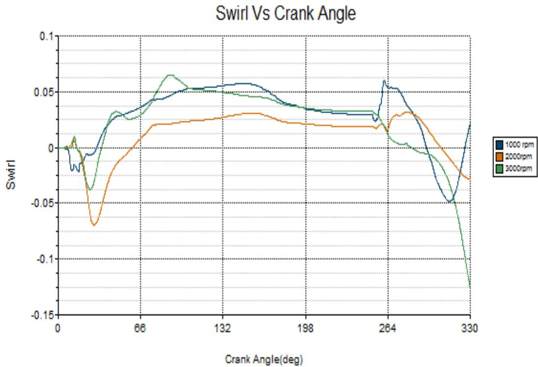
Figure 19. (a) Variation of Swirl with respect to crank angle at Various speed.
