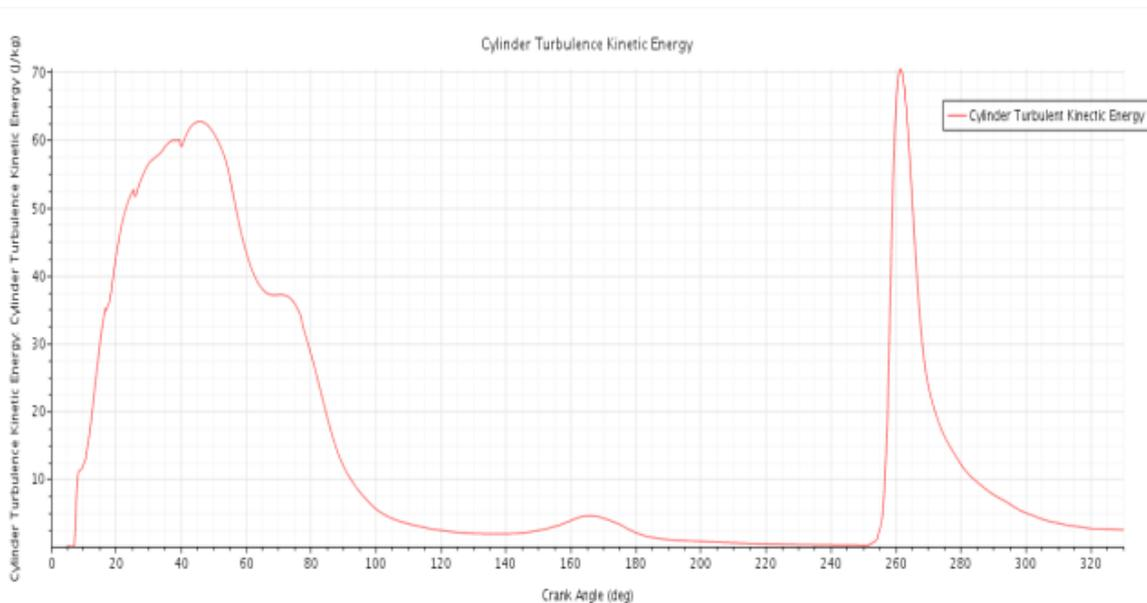
**Figure 18. (d)** turbulent kinetic energy vs crank angle at 3000 rpm.
