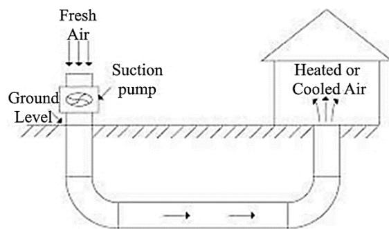
**Fig. 1.** Earth tube heat exchanger flow diagram.
