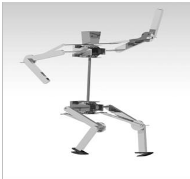
Fig. 9: The Conventional Robot Consisting of only Legs Housing Ten Actuators.
