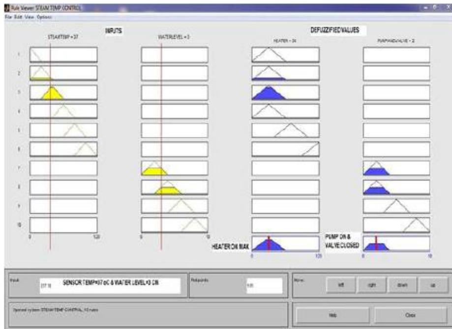
Fig. 10: Simulated Output when Steam Temp=37°C and Water Level=3 cm.
