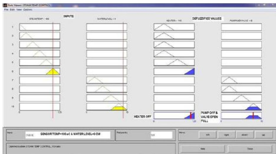
Fig. 11: Simulated Output when Steam Temp=100°C and Water Level=9 cm.
