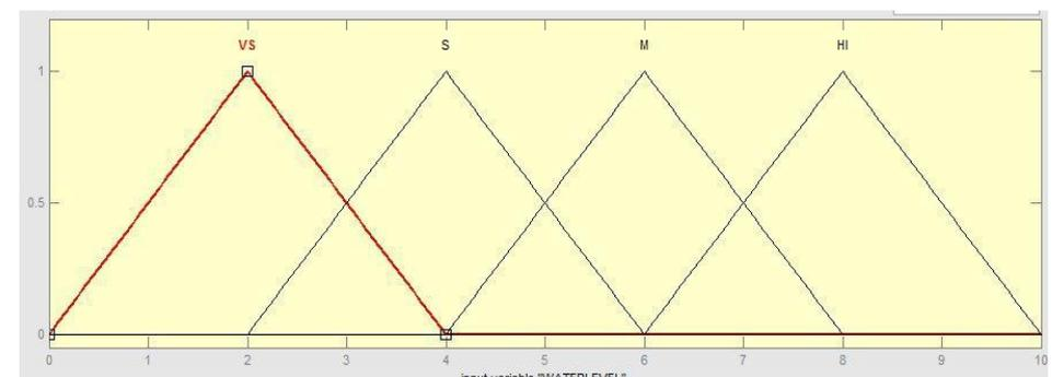
Fig. 8: Input Membership Function: WATERLEVEL.
