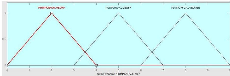
Fig. 9: Output Membership Function: PUMPANDVALVE.
