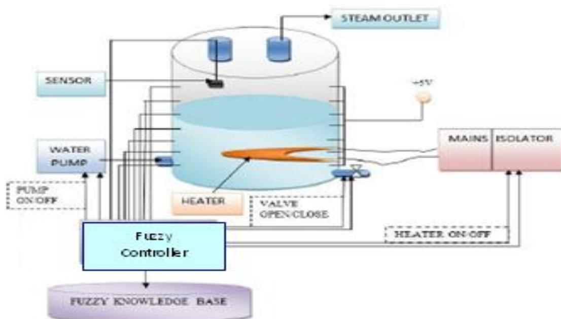
*Fig. 1: Proposed FLC Based Boiler Control System.*
