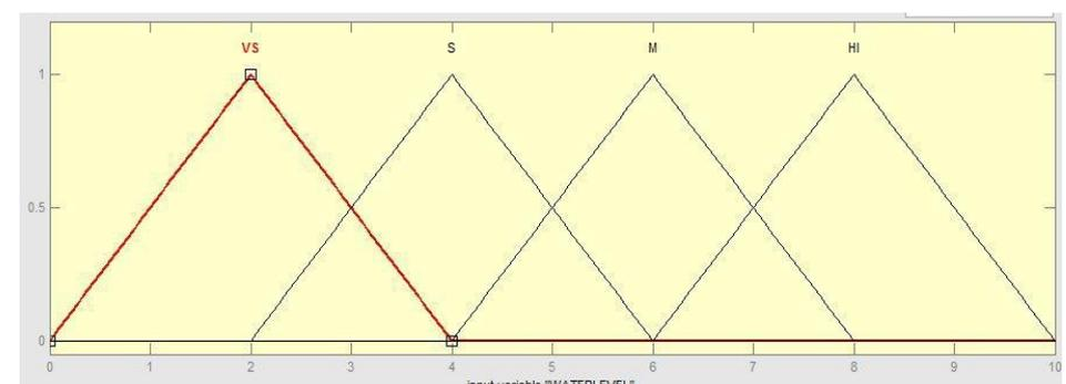
Fig. 8: Input Membership Function: WATERLEVEL.
