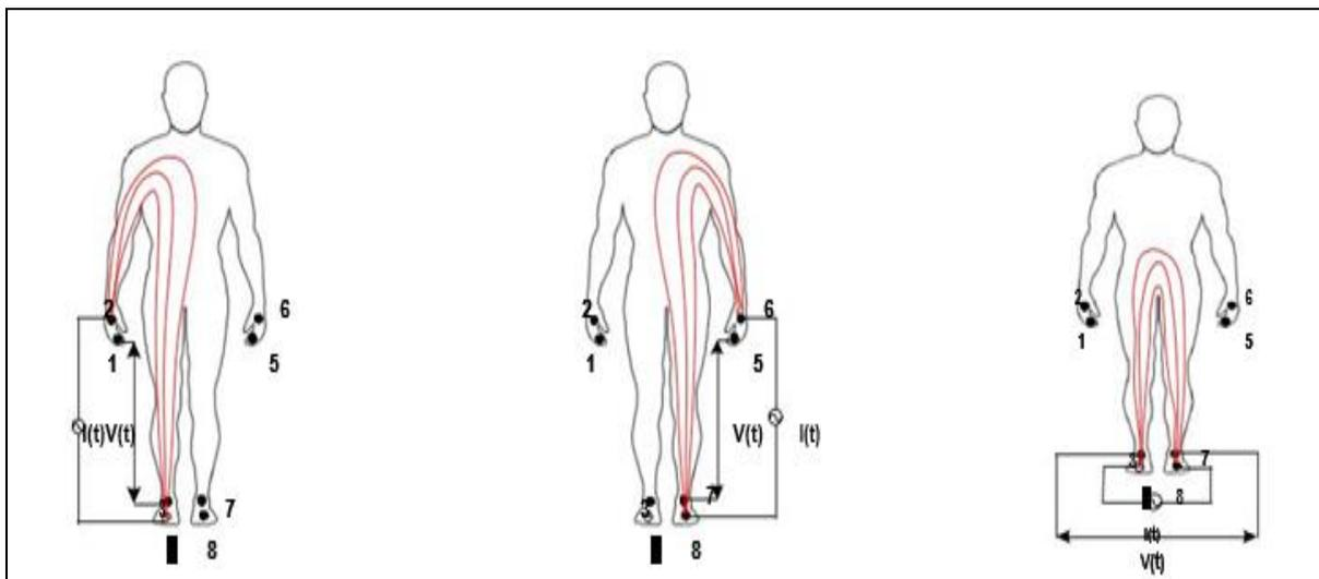
Fig. 2. Electrodes Distribution and the Current Flowing Through Body.
